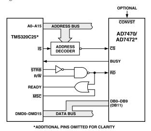
Figure 19. Interfacing to the TMS320C25
