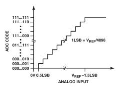
Figure 6. Transfer Characteristic for 12 Bits
