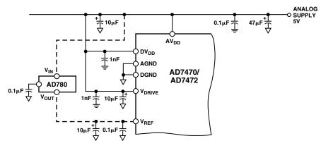
Figure 16. Decoupling Circuit
