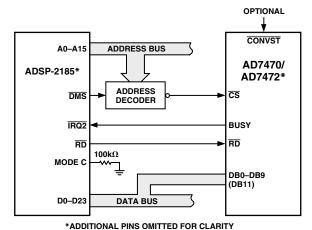
Figure 17. Interfacing to the ADSP-2185
