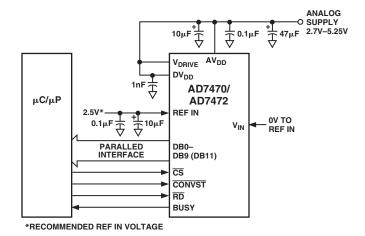
Figure 5. Typical Connection Diagram
