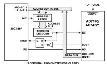
Figure 21. Interfacing to the 80C186
