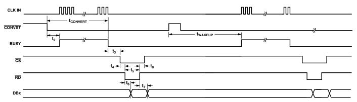
Figure 12. Wake-Up Timing Diagram (Burst Clock)
