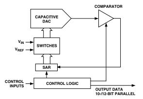
Figure 2. Simplified Block Diagram of AD7470/AD7472
