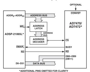
Figure 18. Interfacing to ADSP-21065L
