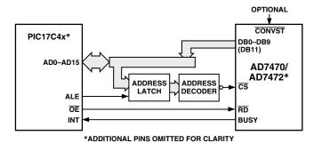
Figure 20. Interfacing to the PIC17C4x
