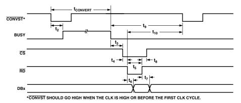
Figure 10. Parallel Port Timing
