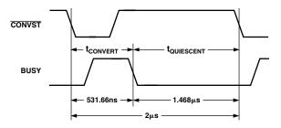
Figure 14. Mode 1 Power Dissipation
